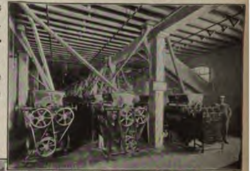
The manufacture of flour at Minneapolis. The wheat is first raised by elevators to the top of the mill, which is usually a building from eight to ten stories in height. After the grain is separated from chaff and seeds, it is thoroughly acoured and prepared for grinding. The first picture shows a grinding room, where the grain is passed between steel or porcelain rollers.
